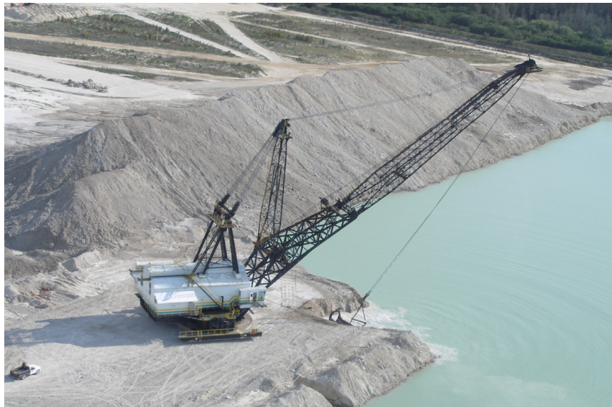
Drag line removes material from quarry pit and allows it to drain before processing.
